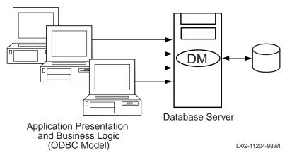
Figure 1–7 Three-Tier Client/Server Environment
